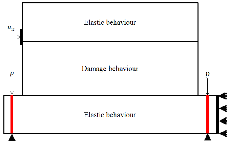
Figure 10. Loading and boundary conditions
