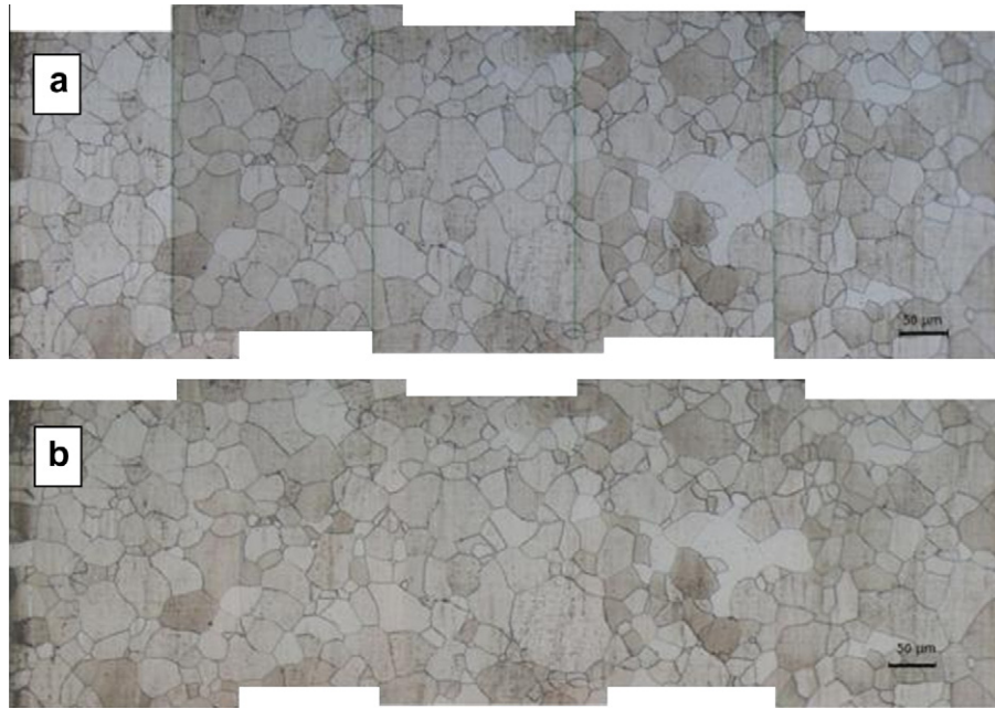
Fig. 9. (a) Before fatigue; (b) micrograph after 5.3 \times 10^9 cycles at 88 MPa.
