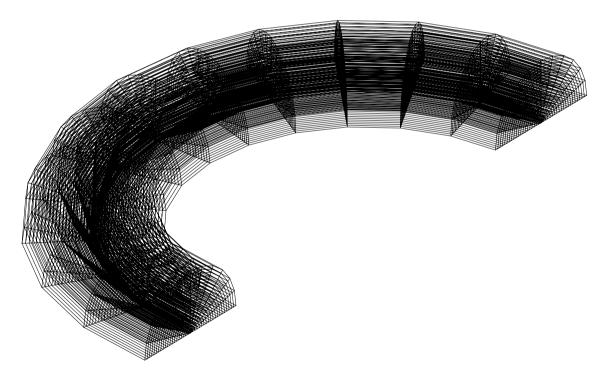
Fig. 6 Finite element mesh around the crack front.
