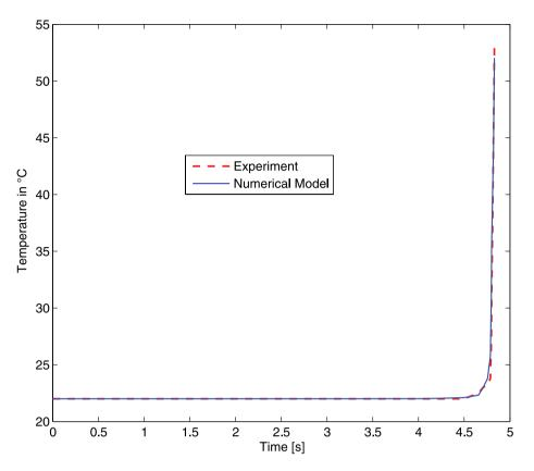
Fig. 8 Test 1: Comparison between the modeled and the experimental temperature during the formation of the fish-eye (initial inclusion 10.03  $\mu$ m, eccentricity 0.79).
