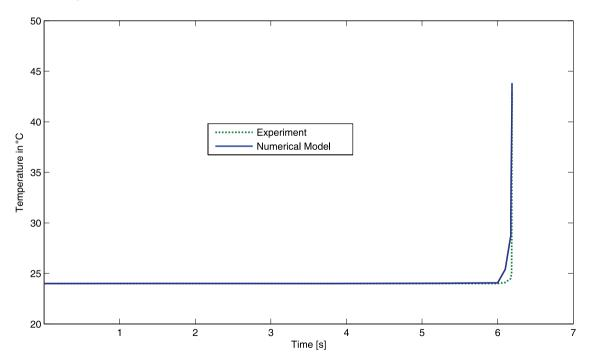
Fig. 9 Test 2: Comparison between the modeled and the experimental temperature during the formation of the fish-eye (inclusion 13.83  $\mu$ m, eccentricity 0.83).
