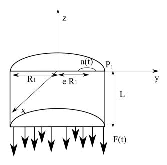
Fig. 2 Model description: one quarter of the cylinder.
