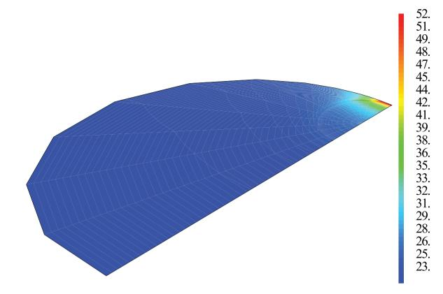
**Fig. 14** Temperature field in  $^{\circ}$ C at t = 4.84 s.
