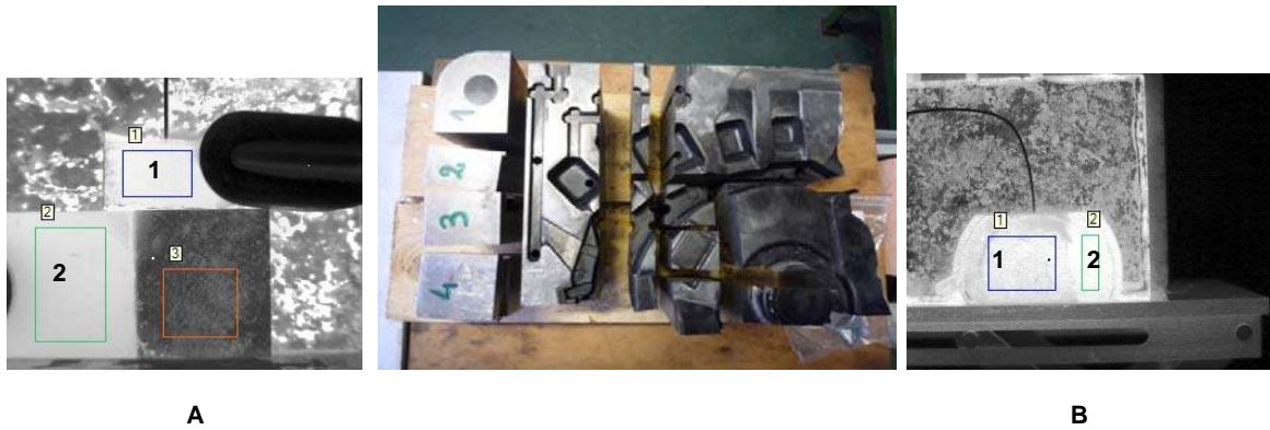
Figure 2 : Two specimens taken from the die surface for the emissivity measuring, A: non- damaged and B: damaged surface
