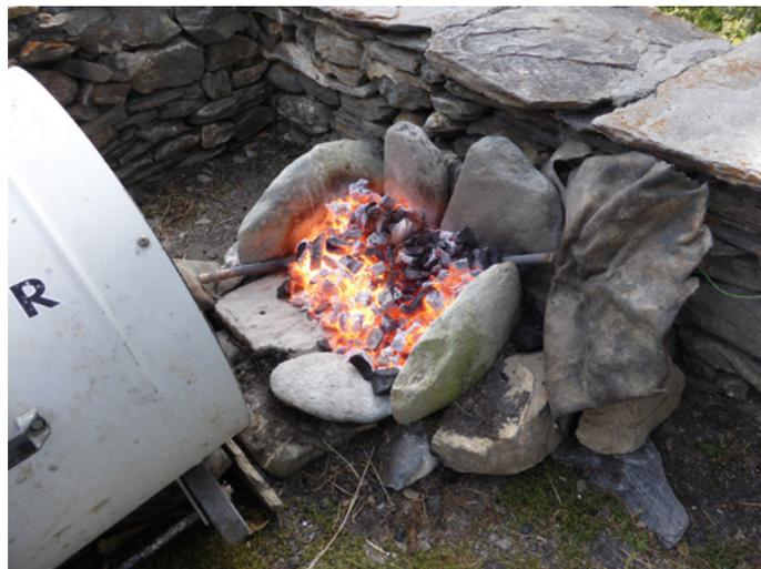
Figure 4b Reconstruction of an Ujina-Collahuasi bench-shape furnace for a smelting experiment; a 40 km/h<sup>-1</sup> wind was produced with an industrial fan.
