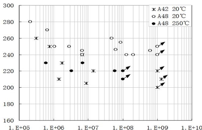
Fig.2 Ultrasonic fatigue test results for specimens tested at 20 and 250°C
