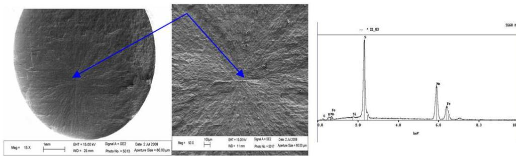
Fig.3 Fatigue crack initiate from interior inclusion (MnS) of A48 steel
