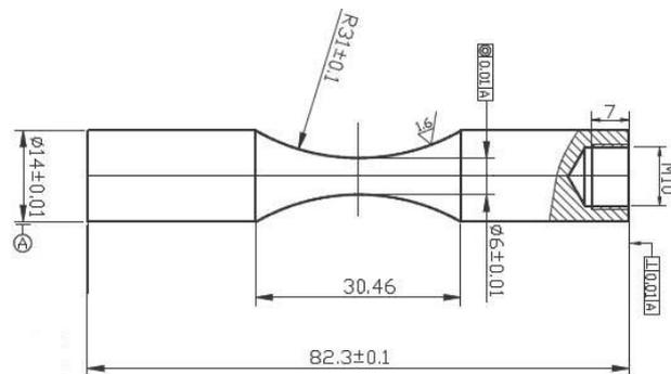
Fig. 1. Ultrasonic fatigue specimen
