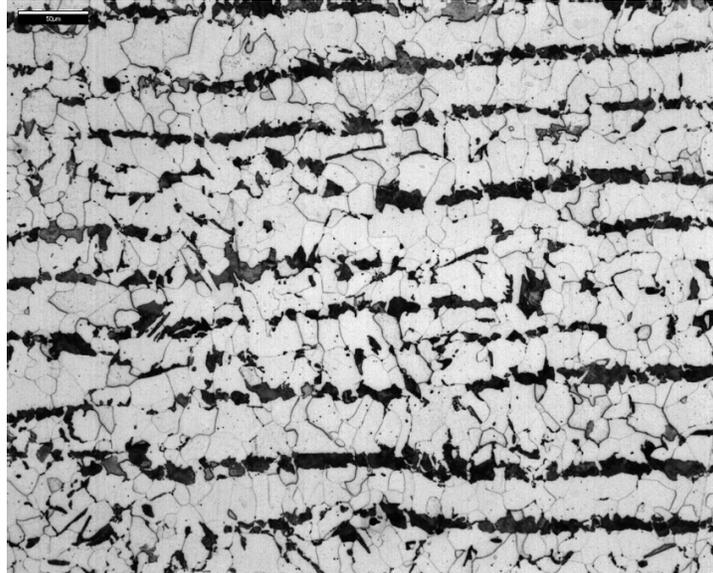
Figure 1 Microstructure of the steel A42
