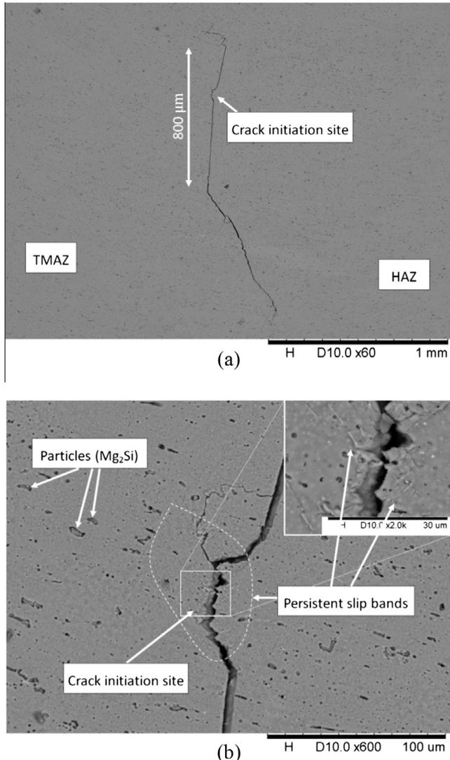
**Fig. 8.** SEM observations of a fatigue crack on specimen surface ( $N_f = 8.74 \times 10^7$  cycles,  $\sigma_b = 70$  MPa). (a) The crack locating between TMAZ and HAZ with whole morphology; (b) enlargement of the fatigue crack initiation site showing persistent slip bands.
