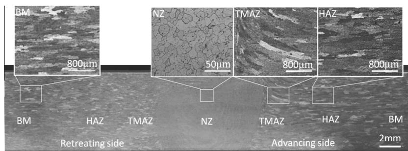
Fig. 2. Metallographic cross-section of the FSW weld.
