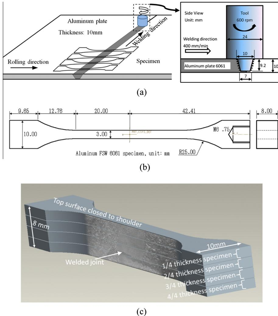
**Fig. 1.** Specimen design of FSW joint in this test. (a) Location of full thickness specimens on the FSW jointed plates; (b) dimensions of full thickness specimen in ultrasonic fatigue test; (c) schematic illustration of the partial specimen through thickness.
