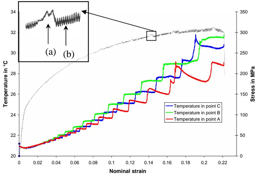
Fig 2. Stress-strain curve and temperature evolution for test 3
