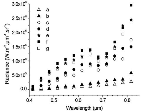
Fig. 6. Radiance spectra at different times for shot 1020: (a) after shock entrance (0.3  $\mu\text{s}$ ), (b) before the superdetonation formation (1.2  $\mu\text{s}$ ), (c) superdetonation formation (1.65  $\mu\text{s}$ ), (d) 1.9  $\mu\text{s}$ , (e) catch-up of the shock wave (2.15  $\mu\text{s}$ ), (f) strong detonation (2.45  $\mu\text{s}$ ), (g) overdriven steady state detonation (3.8 to 4.4  $\mu\text{s}$ ). Radiance values were averaged around the given time value.
