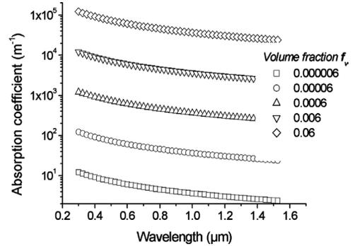
Fig. 17. Absorption coefficient of carbon clusters with varying volume fraction according to Rayleigh scattering.
