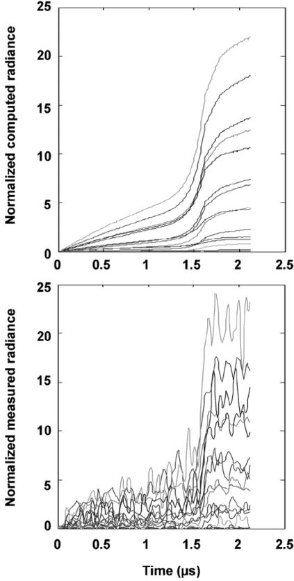
Fig. 13. Comparison of the computed (retrieved) radiance and the measured radiance profiles during SDT.
