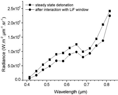
Fig. 10. Comparison of the radiance spectra before and after the interaction with the LiF window.
