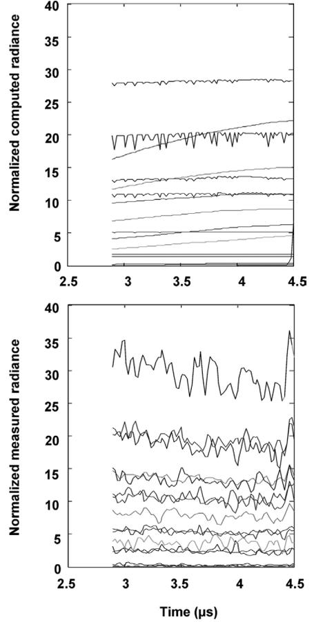
Fig. 14. Comparison of the measured radiance and the computed radiance profiles during the propagation of the detonation.
