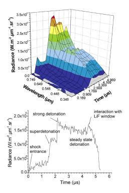
Fig. 4. 3D radiance profiles of shot 1020 and one typical temporal profile.
