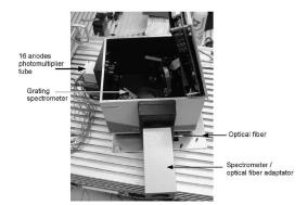
Fig. 3. Emission spectroscopy device.
