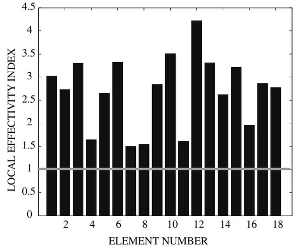
Fig. 10. Local effectivity indexes in the elements in order of increasing stresses.
