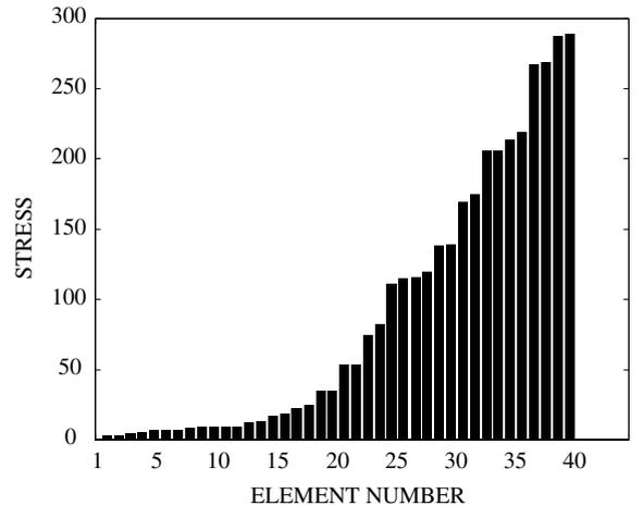
Fig. 3. Local stress density per element in order of increasing stresses.
