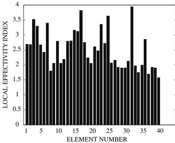
Fig. 5. Local effectivity indexes in elements in order of increasing stresses.
