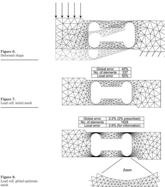
Figure 8. Load cell: global-optimum mesh
