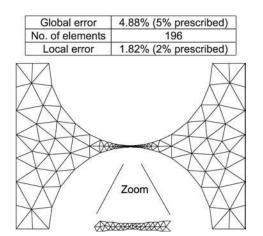
Figure 14. Connection: local-optimum mesh
