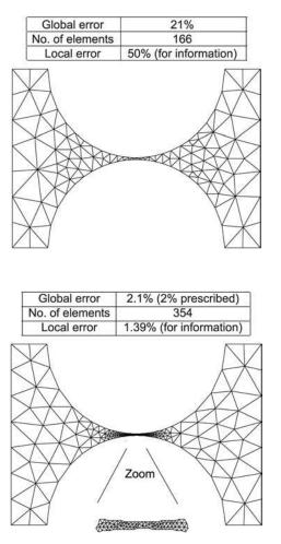
**Figure 12.** Connection: initial mesh
