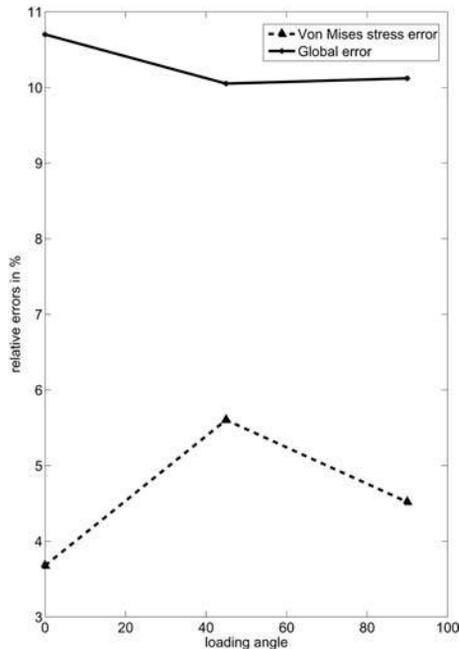
**Figure 14.** Estimated local errors vs the global energy error estimator for the initial problem
