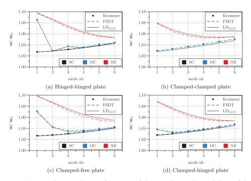
**Figure 3.** T1: Ratio between the eigenfrequencies of the piezoelectric plate and those of the equivalent elastic plate for different mechanical boundary conditions and electric circuits.
