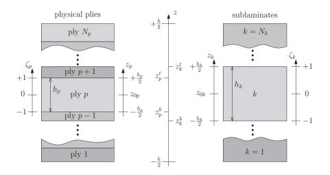
Figure 1. SGUF: geometry description and employed coordinates across the thickness.
