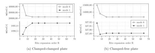
Figure 2. T1: Convergence analysis for first and sixth eigenfrequencies of the CC and CF plate.
