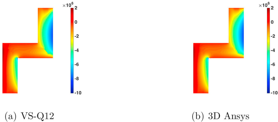
Fig. 18. \sigma_{13}(x = 0, y, z) - Z-shaped beam.
