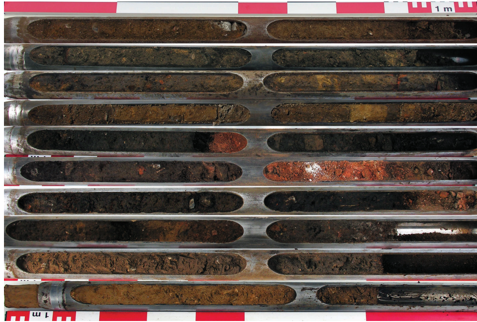
Figure 4.4. Assemblage of the successive parts of Core C1, Taken With the Open-Gauge Method
