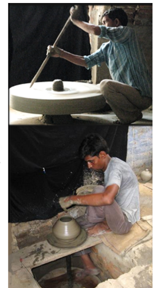
Fig. 2. The two common wheels used in northern India. Top panel: the high inertia stick-wheel used by the Prajapati potters. Bottom panel: the low-inertia kick-wheel used by the Multani potters. Drawings are adapted from Orton et al. (1993). The two wheels evoke distinct body positions: for the stick-wheel potters typically squat (sometimes they use a low stool), while for the kick-wheel potters sit, one leg folded, on a wooden plank.
