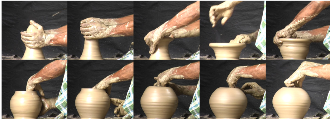
Fig. 1. Example of successive hand positions used during wheel-throwing. The images were extracted from a video recording of an Indian Multani potter throwing a 2.25 kg sphere.
