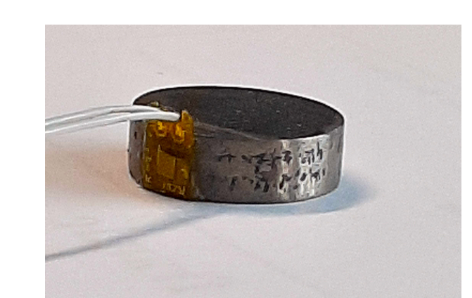
Small strain gauge (size 5x4 mm 2 ) on Ni pellet
