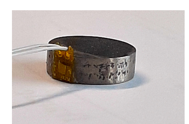
Small strain gauge (size 5x4 mm 2 ) on Ni pellet
