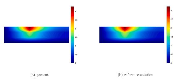
Fig. 10. Distribution of temperature over the beam at  $t = t_{max}$  · NC = 3 layers -  $I_3 = [0.38, 0.4]$  - heat source in layer 3.
