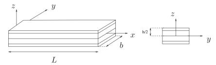
Fig. 1. The laminated beam and coordinate system.
