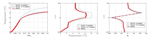
Fig. 14. Multi-resolution ( $T_z$ , then  $T_t$  updated) - initial configuration: 3 layers with a heat source in layer 2 - final configuration: 6 layers with a heat source in layer 4 -  $I_1 = [0.3, 0.4]$  - ramped.
