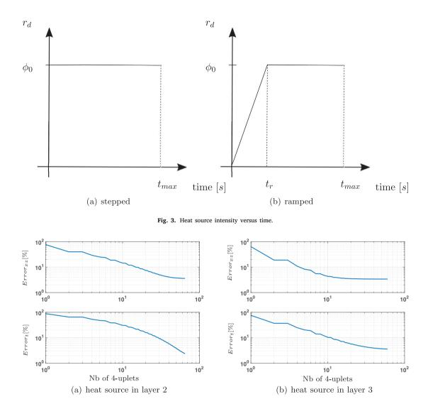
Fig. 4. Error rate with respect to the number of 4-uplets - NC = 3 layers -  $I_3 = [0.38, 0.4]$  - heat source in layer 2/3.
