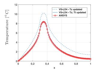
**Fig. 15.** Multi-resolution ( $T_z$ , then  $T_i$  updated) - initial configuration: 3 layers with a heat source in layer 2 - final configuration: 6 layers with a heat source in layer 4 -  $I_1 = [0.3, 0.4]$  - ramped.
