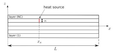
Fig. 2. The laminated beam and heat source.
