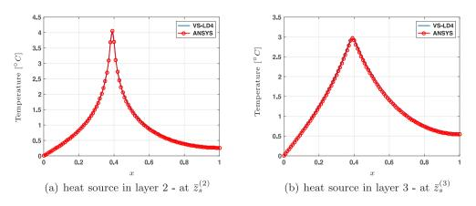
Fig. 5. Distribution of temperature along the beam length -  $t = t_{max}$  - NC = 3 layers -  $I_3 = [0.38, 0.4]$  - heat source in layer 2/3.
