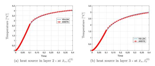
Fig. 8. Distribution of temperature with respect to the time - NC = 3 layers -  $I_3 = [0.38, 0.4]$  - heat source in layer 2/3.
