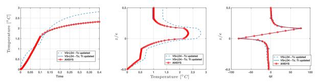
Fig. 18. Multi-resolution ( $T_2$ , then  $T_1$  updated) - initial configuration: 3 layers, constant heat source in layer 2 - final configuration: 6 layers, heat source in layer 4 with stepped time variation -  $I_2 = [0.38, 0.4]$ .
