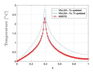
**Fig. 19.** Multi-resolution ( $T_z$ , then  $T_t$  updated) - initial configuration: 3 layers, constant heat source in layer 2 - final configuration: 6 layers, heat source in layer 4 with stepped time variation -  $I_2 = [0.38, 0.4]$ .
