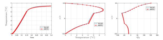
Fig. 11. Multi-resolution (only  $T_t$  updated) - ramped  $t_r = 0.15$  s - 3 layers -  $I_3 = [0.38, 0.4]$  - heat source in layer 3.
