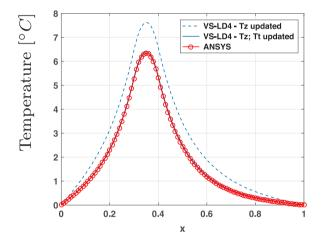
**Fig. 13.** Multi-resolution  $(T_z, \text{ then } T_t \text{ updated})$  - initial heat source in layer 2–3 layers -  $I_3 = [0.38, 0.4]$  - heat source in layer 3 - ramped.
