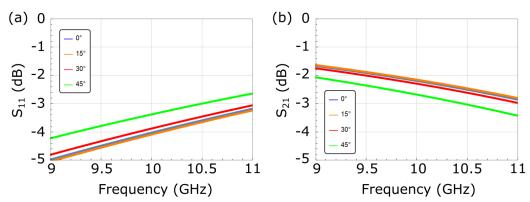
**Figure 2.** Evolution of the S-parameters of the optimized unit cell as a function of frequency for  $0^{\circ}$ ,  $15^{\circ}$ ,  $30^{\circ}$ , and  $45^{\circ}$  obliquely incident illuminations. (a)  $S_{11}$  and (b)  $S_{21}$ . The S-parameters are obtained by simulating the optimized unit cell with Floquet ports and periodic boundary conditions.
