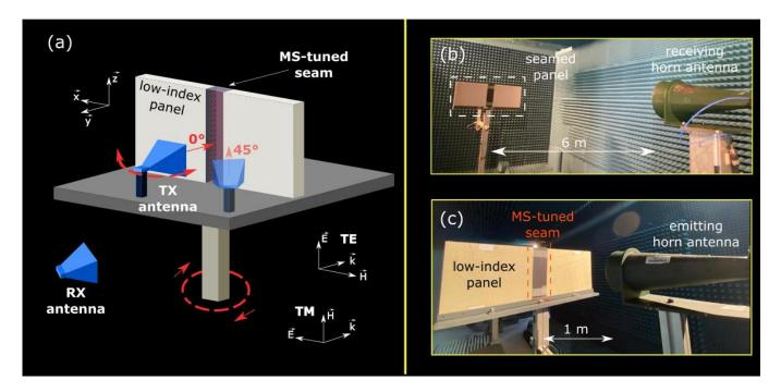
**Figure 4.** (a) Schematic illustration of the studied structure. Two low-index radome panels are connected via a high-index MS-tuned seam. The structure is illuminated by an emitting (Tx) antenna and a receiving (Rx) antenna allows us to measure the antenna radiation patterns for different angles of incidence. (b) Photography of the far-field measurement setup in an anechoic chamber. (c) Close up of the emitting antenna illuminating the seamed panel.
