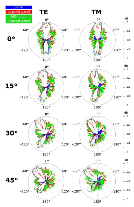
**Figure 5.** Measured far-field radiation patterns in the case of the reference panel (blue), the seamed panel without MSs (red) and the MS-tuned seamed panel (green), for  $0^{\circ}$ -,  $15^{\circ}$ -,  $30^{\circ}$ -, and  $45^{\circ}$ -incident, TE- (**first column**) and TM-polarized (**second column**) illuminations at 10.5 GHz.
