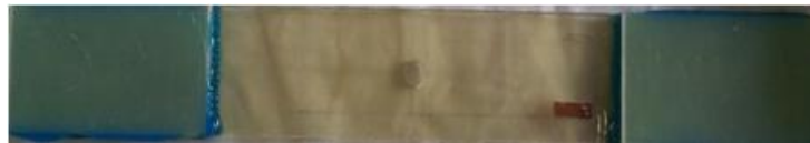
(b) Rectangular specimen with 5 mm in diameter of hole at its center
